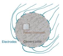
Non-destructive EIT-based corrosion detection:
